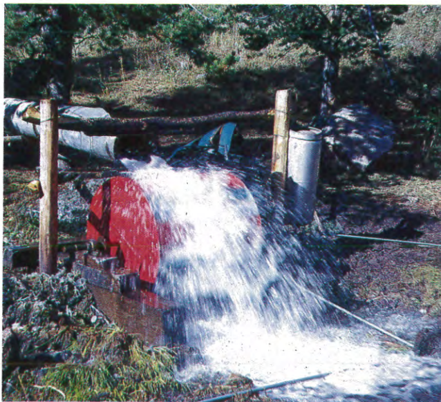
An overshoot water wheel on the Beaverhead National Forest uses the power of falling water to pump water to higher elevation rangeland, allowing grazing by both domestic livestock and wildlife on otherwise waterless rangeland.
